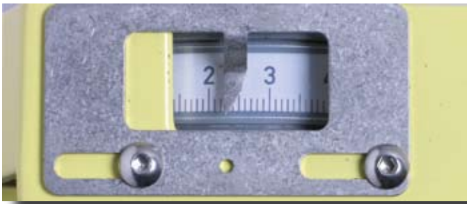
Level reading on high accurate graduated tape +/- 1.5 mm over 30 meter
